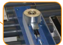
Self-tensioning & tracking side drives simplify belt replacement
